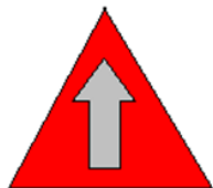
Fire Hose Connection
