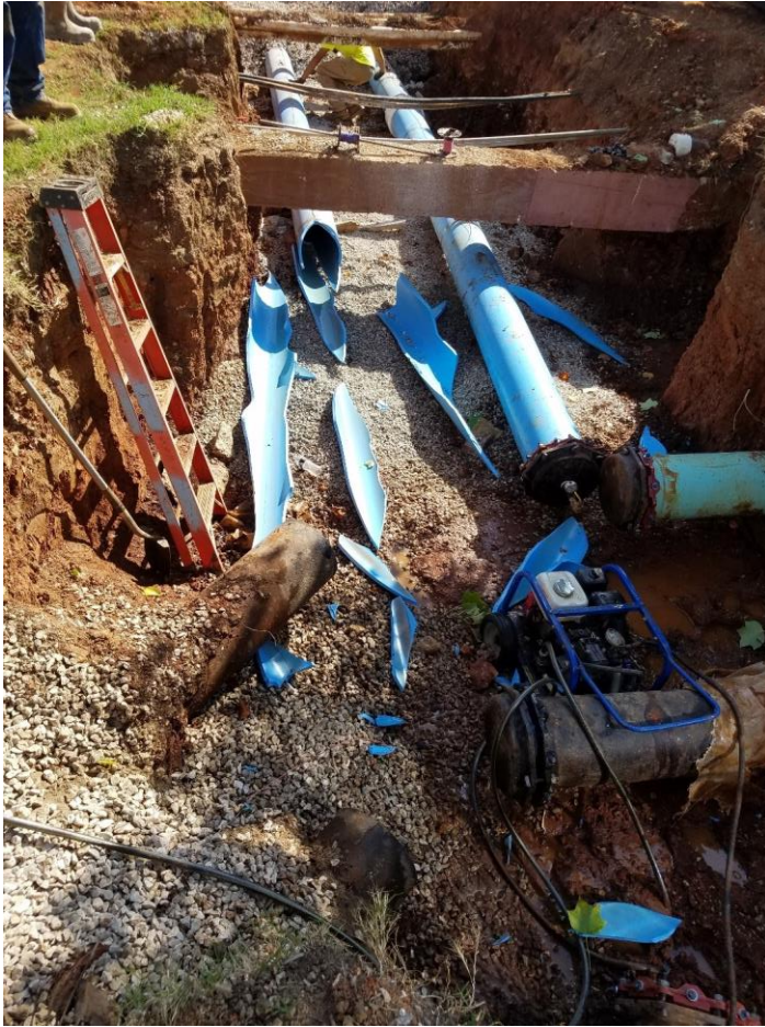
Figure 2: Failed section of 12" C-900 Chilled Water Piping.
